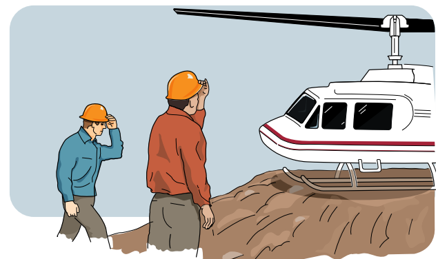
Figure 50-11 Approach or leave on the downslope side
